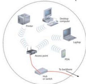
Figure 3-41: An infrastructure WLAN
