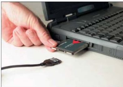
Figure 5-11: Installing a PCMCIA-standard NIC
