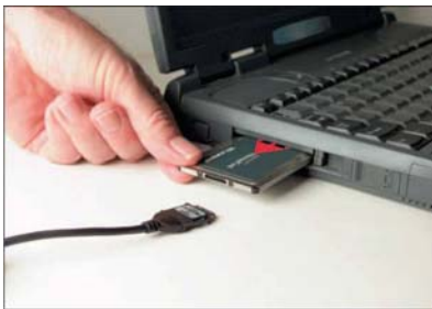
Figure 5-11: Installing a PCMCIA-standard NIC
