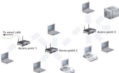
Figure 6-17: A WLAN with multiple access points
